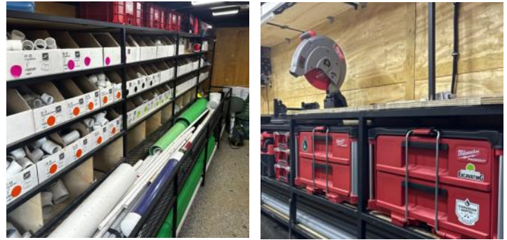
Pipe racks installed on the lower portion on both sides of the work trailer, with shelving and a trough above that on one side. The setup also includes a work bench with plenty of storage for extra batteries.
